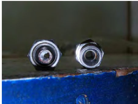
Figure 1.3: The scaling of an untreated pipe (left) compared to a pipe treated with Hydropath (right) (page 10).
