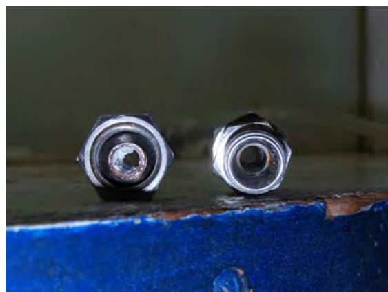
Untreated Tube (left) Treated Tube (right)
